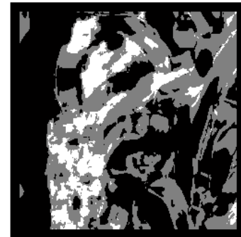
Fig. 1 Region characterization for image Lena: black – flat region, gray – moderate busy regions, and white – busy regions.
