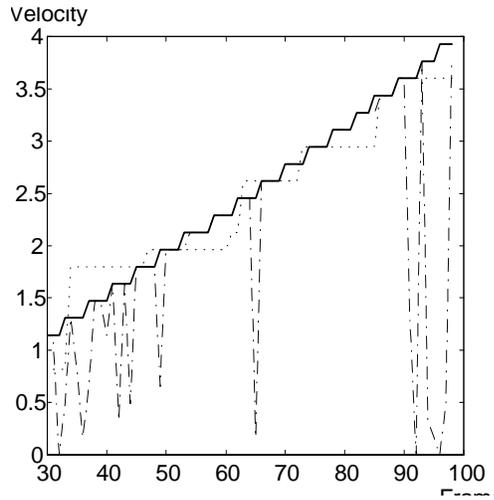
Figure 6: Velocity estimation in the noisy case, based on: Spectrogram (dotted line); Wigner distribution (dashed line) and local polynomial periodogram (solid line).
