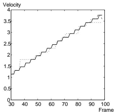
Figure 3: Velocity estimation based on: Spectrogram (dotted line), Wigner distribution (dashed line) and local polynomial periodogram (solid line).
