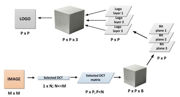
Fig. 2. Scheme of logo extraction procedure
