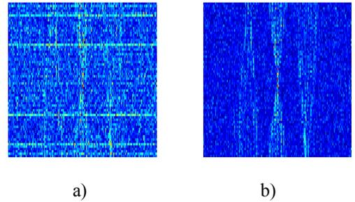
Fig. 2. a) Standard Ambiguity function of a noisy signal b) L-form of the Ambiguity function
