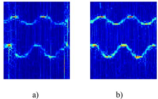
Fig. 3. Choi-Williams distribution calculated using: a) Standard Ambiguity function b) L-form of the Ambiguity function.
