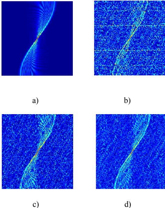
Fig. 1. Non noisy case: a) Ambiguity function; Noisy case: b) Ambiguity function of the noisy signal c) Median form of the Ambiguity function d) L-form of the Ambiguity function
