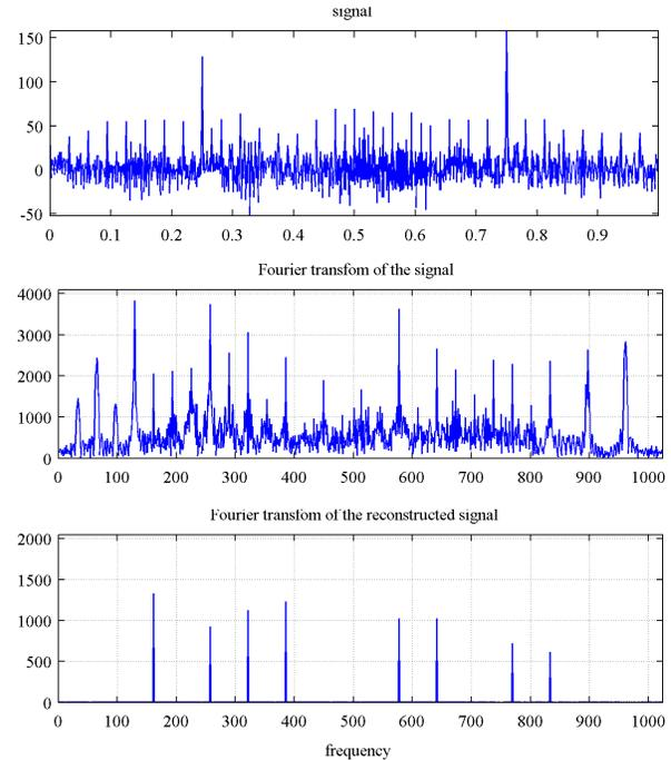
**Fig. 4.** Signal composed of a sparse part and non-stationary part, with additional transient impulses in time, including two strong pulses (top), Fourier transform of the original composite signal (middle). The reconstructed Fourier transform by using the CS values of the STFT, corresponding to sparse part of the composite signal (bottom)
