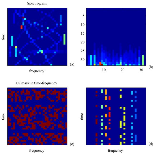
**Fig. 3.** a) STFT of the composite signal, b) Its sorted values, c) CS mask corresponding to the L-statistics based STFT values, d) STFT values that remain after applying the L-statistics on the absolute values of the STFT (bottom)
