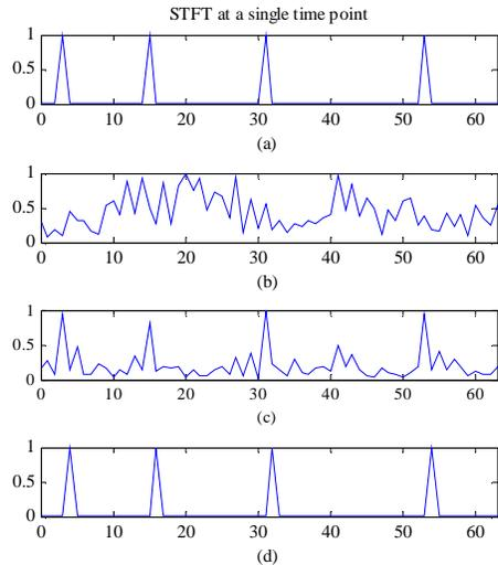
**Fig. 1.** a) STFT of non-noisy signal, b) STFT of noisy signal, c) L-estimate STFT, d) CS L-estimate STFT
