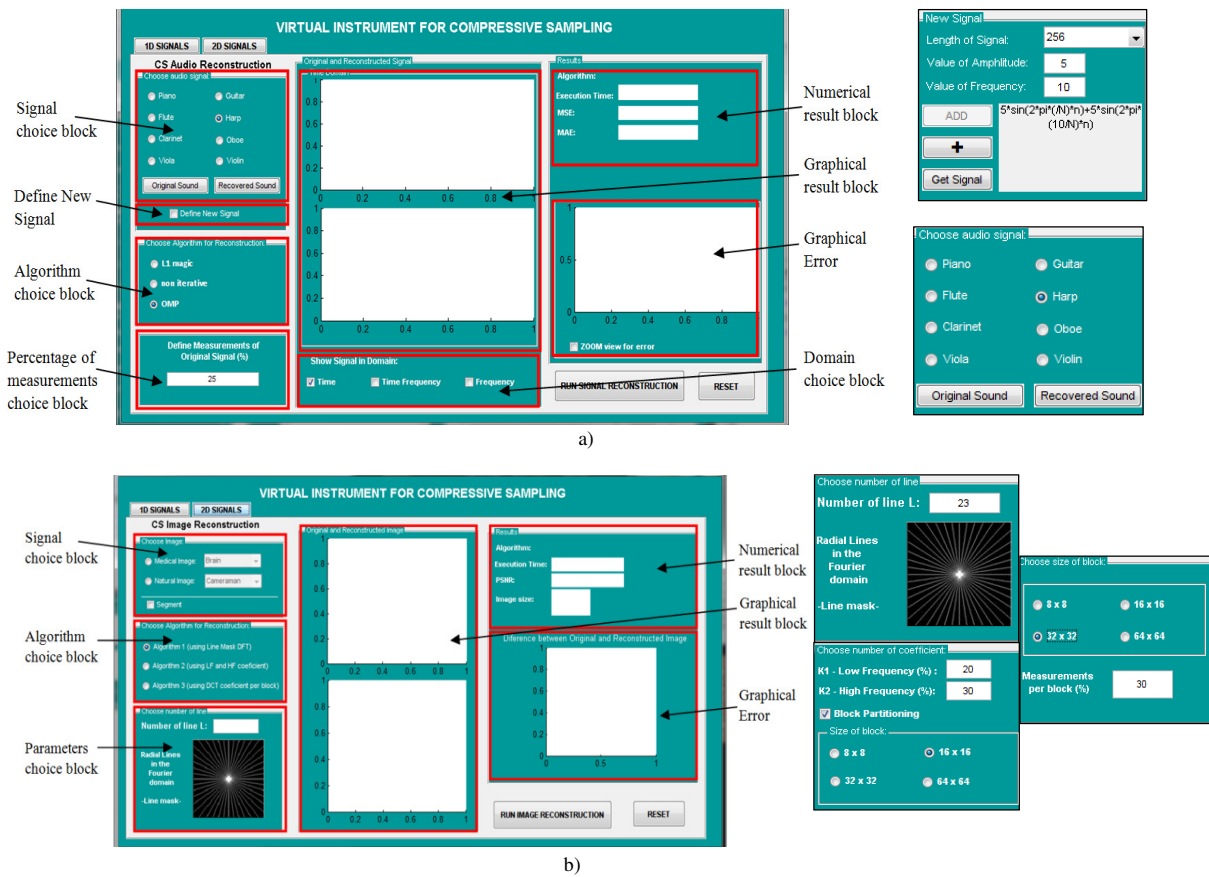
Fig. 1. The outlook of the proposed Virtual Instrument (for 1D and 2D signals)
